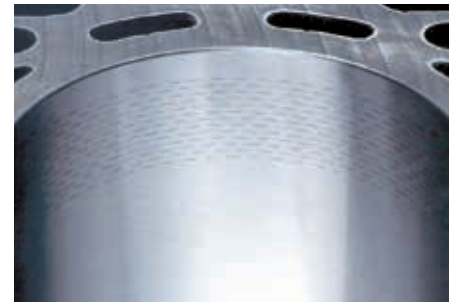
Cylinder bore after laser honing
