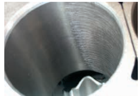
Cylinder bore, left side of picture: Boring position before honing, right side of picture: Boring position at the start of position honing
