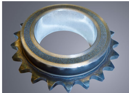
Chain wheel (front face connection)
